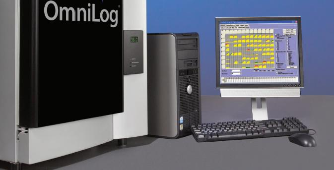
Biolog's OmniLog enables high throughput, automated kinetic cell assays on 50 microplates (4,800 wells) at a time. The instrument can be used with Biolog's preconfigured PM phenotypic assay panels or with any other colorimetic assays. Microplates are read in place. They do not have to be moved to a reader and the lids do not have to be removed during reading, preserving sterile incubation conditions.
