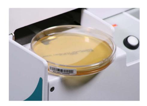
The unit automatically tags barcode labels on the side walls of Petri plates.
